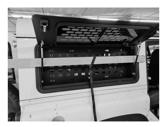
3. Then clamp the Expedition box on the inside of the window vertically in two places with a clamping tong.
